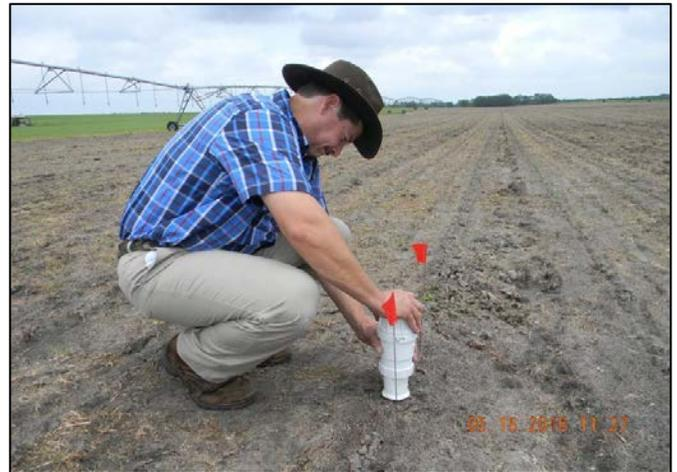
*Once installed, only the head of the probe is exposed. Information is transmitted through cellular signals to the farmer.*
